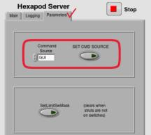
Note: If the GUI is used after being set to DDS mode, the system will switch back the Command Source to GUI and ignore any DDS commands. The Command Source must show DDS in order to receive DDS commands.
