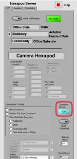
If the Command Source does not show DDS, go to the Parameters tab, select DDS under the Command Source and click the Set Cmd Source button.
